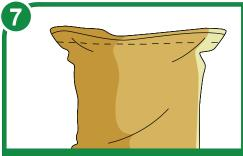
Close the outer bag by tying or sewing at 3cm distance from "zipped" inner liner.
