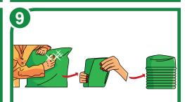
After using, clean, dry and fold undamaged GrainPro Hermectic Bag Premium, and save the reusable cable tie for future use.
