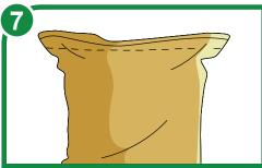
Close the outer bag by tying or sewing at 3cm distance from the "tied" inner liner.
