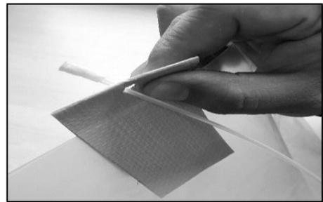
8.3.4. Secure the bottom of the liner and add additional woven OPP tape aligned in container hooks. Insert the nylon rope into the woven OPP tape and tie it to the hooks.
