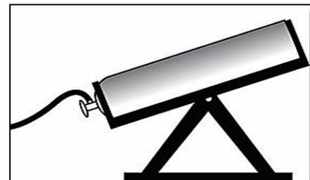
c) If a mechanical inverter is not available, a makeshift inverter can be made using sandbags or other improvised techniques. The cylinder should be inverted with its top resting on one sandbag and the bottom end resting on a pile of two or three sandbags high.
