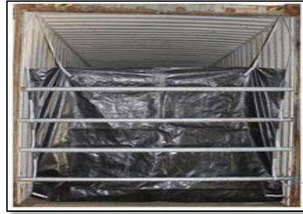
8.11.3. Pull the ends of the TSL™ Bulk zipper for sealing.
