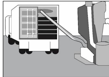
8.7.5. Make sure to leave at least 20 cm. of space between the roof of the container and the top of the commodity to prevent condensation.
