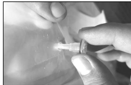
8.10.4. Screw the plastic valve body. The cap of the plastic valve should be positioned outside the loaded TSL™ Bulk.
