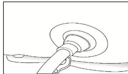
8.12.4. Twist the plastic valve cap to open.
