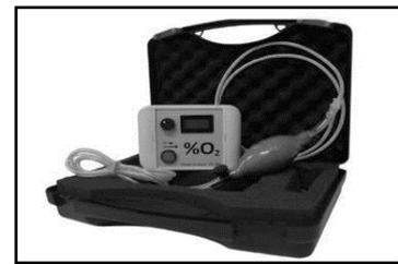
b. Using the analyzer, the oxygen level can be checked through the plastic valve with a flexible adapter hose before unloading. Decreased oxygen level indicates the absence of any source of leaks from punctures, holes, or damages. The oxygen level of ambient air is 20.9%.
