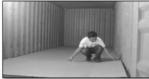
8.1.5. Carefully unfold the TSL™ Bulk. Lay TSL™ Bulk with the broken line markings facing upward.
