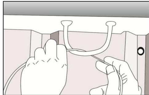
8.3.3. Insert the free end of the nylon rope into the first woven OPP tape. The woven OPP tape in the TSL™ Bulk should be positioned in-between the hooks (except for the first woven OPP tape near the TSL zipper)
