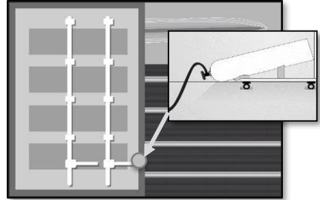
e) Open the cylinder valve. Adjust the opening of the valve until the sound of liquid passing through the hose is observed. The liquid CO<sub>2</sub> flushes into the TSL Bulk and will push the air upward starting from the bottom, creating a piston effect, until the air is totally replaced. The opening through the zipper will serve as an outlet for the displaced air.
