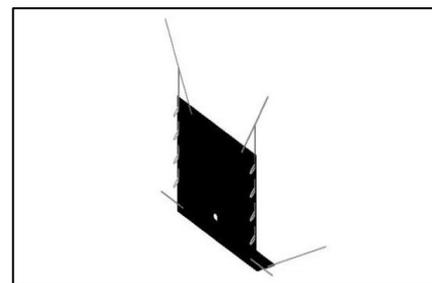
8.4.4 Install four (4) GI pipes (NOT INCLUDED in the TSL™ Bulk Package) for support, 0.4 m apart.
