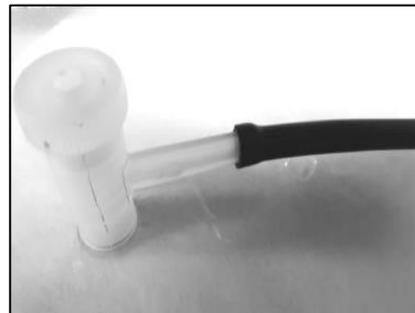
8.13.4. Twist the plastic valve cap to open. Connect the O<sub>2</sub> or CO<sub>2</sub> analyzer to the flexible adapter hose and the reading.
