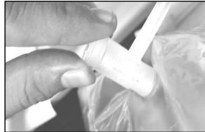
8.12.6. After conducting the PDT, twist the plastic valve to close.
