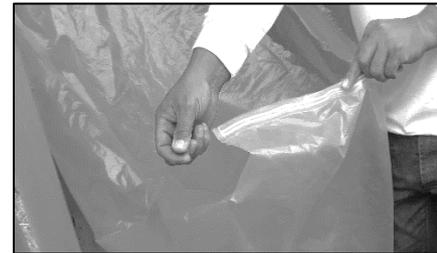
b) Position the slider on the manually zipped portion of the zip lock.
