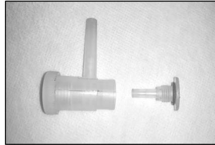
8.10.3. Pierce the TSL™ Bulk using the plastic valve base. Piercing is done from the inner side of the TSL (approximately 20 cm from the zipper).
