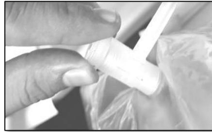
8.13.5. After taking the oxygen or carbon dioxide reading, twist the plastic valve cap to close.
