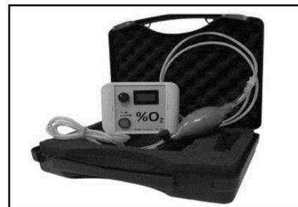
c. Using the analyzer, the oxygen level can be checked through the TSL's plastic valve with a flexible adapter hose.
