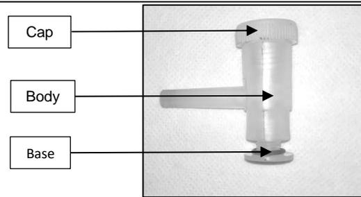
8.10.2. Disassemble the plastic valve by unscrewing the base.
