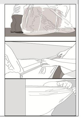
b) Insert and position the slider on the manually zipped portion of the zip lock.
