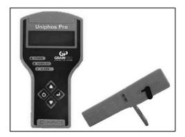
b. Succeeding monitoring should be done twice a week. Carbon dioxide levels should increase to a level greater than 10%. Carbon dioxide level may go up to 15% or more. When decrease in CO<sub>2</sub> level is observed, sealing is probably compromised, and the commodity may not be adequately protected.
