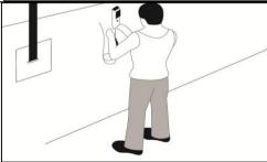
7.7.3 When carrying-out a CO<sub>2</sub> treatment, the approximate CO<sub>2</sub> concentrations can be determined by measuring CO<sub>2</sub> concentrations using the carbon dioxide analyzer.
