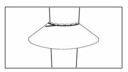
8.4.4 Lock the overlap using staple wire, cable wire, or any fastener.
