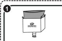
The SGB\*High Capacity comes in a set of hermetic liner and Flexible Intermediate Bulk Container (FIBC). Check SGB\*High Capacity for holes and tears before using. Insert the liner inside the FIBC all the way through the downspout.
