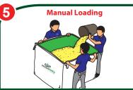
Pour the commodities gently into the hermetic liner. Make sure there is no spillage in between the liner and the bag.
