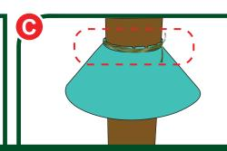
1. To hold the rodent guard in place, Cable tie(A), GI wire (B), or string (C) can be used. Tie the teeth of the rodent guard on the leg using any available fastener.
