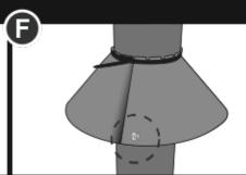
2. The overlap at the bottom can be fastened using staple wire (D), paper clip (E), or small nail/rivet (F).
