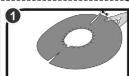
If the leg perimeter is smaller, the rodent guard can be cut in half to fit. Cut along the lines at the back of the rodent guard.
