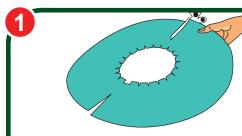
If the leg perimeter is smaller, the rodent guard can be cut in half to fit. Cut along the lines at the back of the rodent guard.
