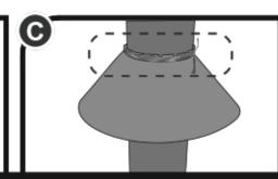
To hold the rodent guard in place, Cable tie(A), GI wire (B), or string (C) can be used. Tie the teeth of the rodent guard on the leg using any available fastener.
