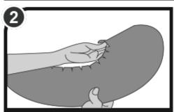
Fold the rodent guard's teeth upwards against the sides of the leg to fit the rodent guard on each leg.
