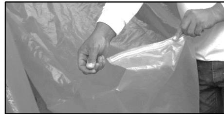
3.3.4. Manually zip a few centimeters on the end of the zipper enough to initially engage the slider.
