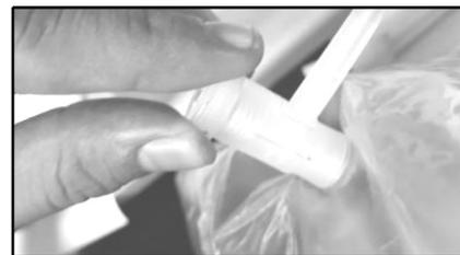
3.5.4. Connect the O<sub>2</sub> or CO<sub>2</sub> analyzer to the flexible adapter hose and the reading. Take readings of CO<sub>2</sub> and O<sub>2</sub> using the available analyzer.
