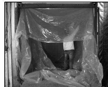
2.1.7. Secure excess liner material near the door perimeter by folding and sticking it on the sides of the door using tapes to prevent possible damage and to make it more accessible during loading.
