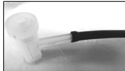
3.4.3. Twist the plastic valve cap to open.
