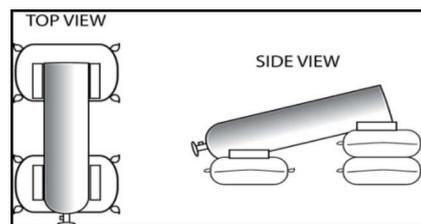
4.3.4. A standard high-pressure hose (available only as separate item) should be connected to the cylinder. This hose should be guaranteed to withstand a pressure of 88 atmospheres (1,300 psi, or 92 kg/cm<sup>2</sup>). Ensure that all connections are made properly, and gaskets are in place where they are required. The high-pressure hose should have a length of about 2-meter and have matching coupler at cylinder.
