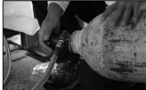
4.3.7. Ice formation along the pressurized hose and the pipe connector during CO<sub>2</sub> flushing:
