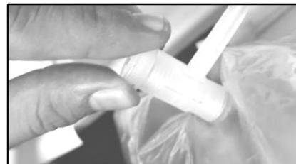
3.4.4. Using a vacuum pump with at least 2.3 cubic meters of suction capacity per minute. Create at least -250 Pascals (Pa) or -25 millimeters' water (mm H<sub>2</sub>O) vacuum inside the TSL by partially opening a portion of the zipper and insert the vacuum pump suction port.
