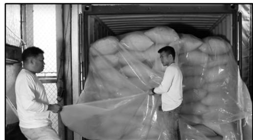
3.3.6. For ease of zipping, two are persons required, one person does the zipping and the other person holds the other end steadily, making sure both sections of the zipper are in a straight line to avoid the zipper length being misaligned. Moving the slider while the zipper or slider is curved forces one of the zipper sections to elongate.
