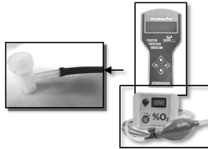
3.5.5. After taking the oxygen or carbon dioxide reading, twist the plastic valve cap to close.
