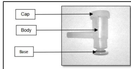
3.2.2. Dismantle the plastic valve by unscrewing the base.
