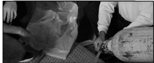
4.3.7.2. Flushing (emptying of the cylinder) depends on the amount of CO<sub>2</sub> to be applied. Emptying one 22kg cylinder should only take about 20 to 30 minutes. If the pressure hose or the inlet valve gets blocked with ice, this is an indication that the CO<sub>2</sub> is being released too quickly. If this happens the cylinder should be closed until the ice melts, and then the cylinder valve should be re-opened and adjusted to reduce the flow.
