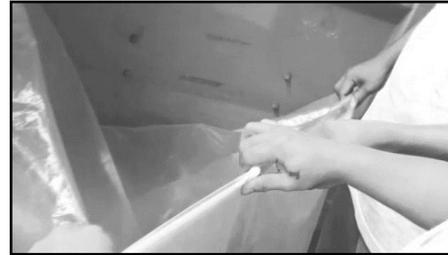
3.3.3. Hold the 2-track zippers together. Aligned for proper sealing.
