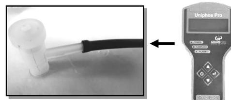
3.6.3. Monitoring of carbon dioxide level is recommended to ensure control of insect infestation. Details of using CO<sub>2</sub> analyzer are discussed in the analyzer's instruction manual.
