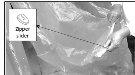
3.3.5. Position the slider on the manually zipped portion of the zip lock.
