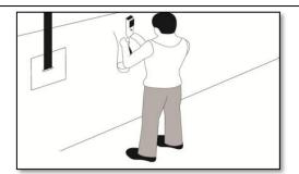
5.8.3. When carrying-out a CO<sub>2</sub> treatment, the approximate CO<sub>2</sub> concentrations can be determined by measuring CO<sub>2</sub> concentrations using the carbon dioxide analyzer.
