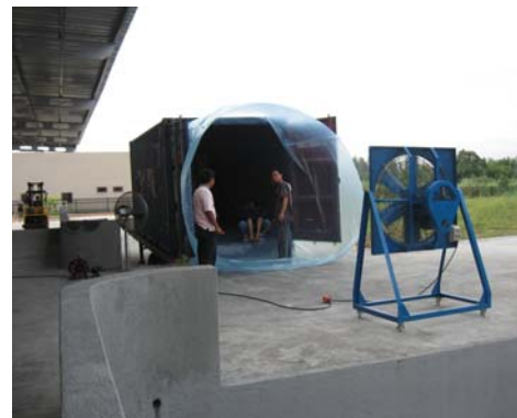
Figure 2. Positioning blower 5 meters away from container
