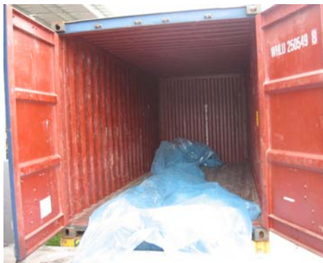
Figure 1. Laying the liner inside the container.
