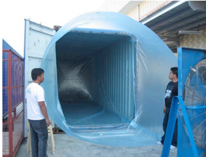
FIGURE 2 – Loading TranSafeliner in standard 20ft. shipping container
