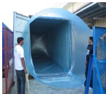
Figure 8: TranSafeliner™ being installed in a transport container, 2008.
